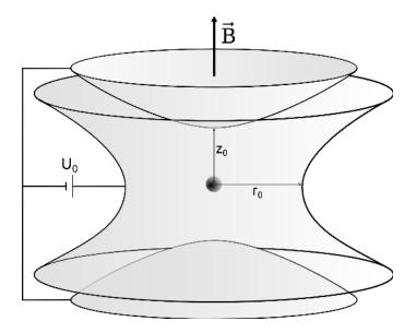
Penning trap. By combining a magnetic field and an electric field, charged particles can be trapped in the laboratory.
